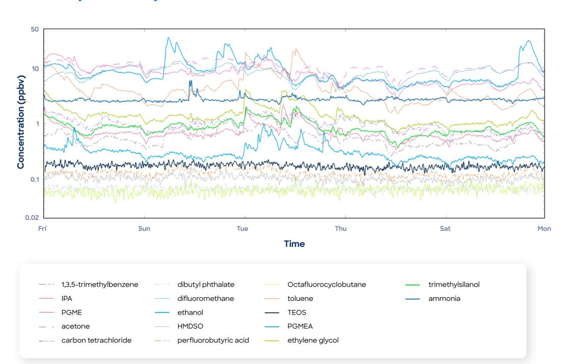
Online AMC monitoring of a diverse range of volatile organic compounds. Detection of AMCs occurred within the lower half of Voice200infinity's dynamic range which extends to low ppt levels.
